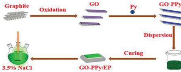
Fig. 5.3: Schematic representation of synthesis of graphene oxide-polypyrrole [50].
